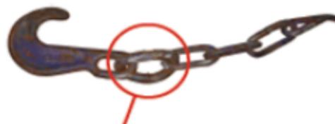
Deformed links / steel parts
