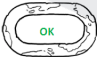
Acceptable level of corrosion
