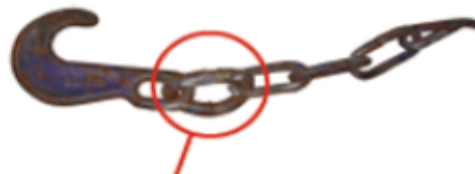
Deformed links / steel parts
