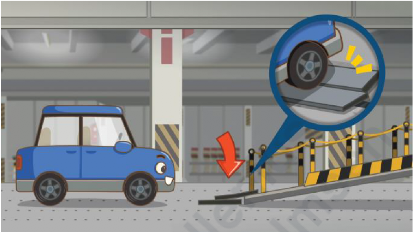
Example of rubber mats on internal ramp
