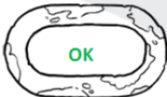
Acceptable level of corrosion
