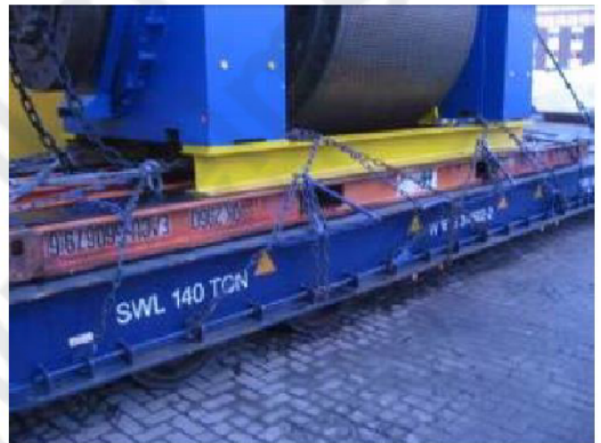
Chain hooks fixed to the base structure of the cargo items
