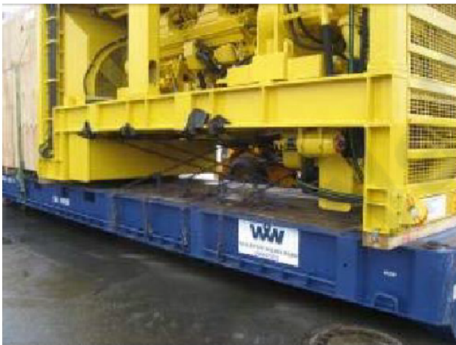
Chain hooks fixed to the base structure of the cargo items
