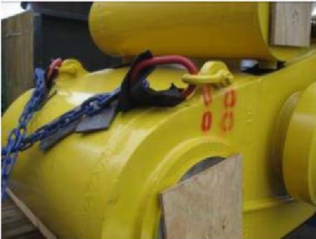
Chain hooks fixed to lashing fittings on the cargo item
