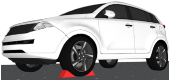
Car with two chocks placed around one front wheel.
